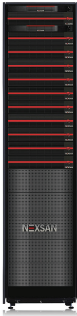
Figure 3 NST6530 with Nexsan NST224X SAS Storage Enclosures in a 42U rack.
